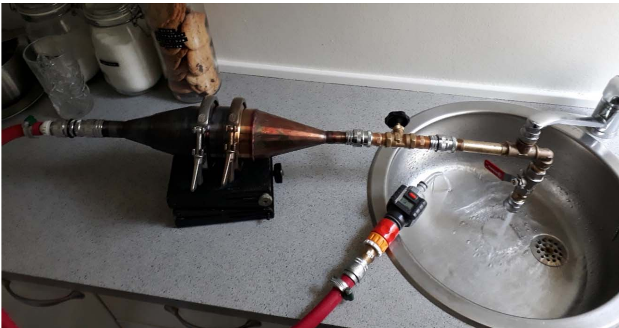
Figure 2. Tap water sampling. Deployment of the stainless steel sampling column to the drinking water tap for collection of 50 L water samples.
